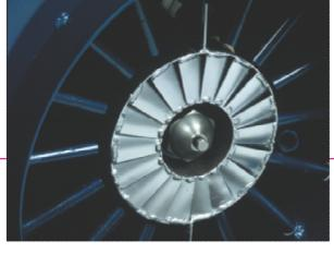
Unique firing head produces stable combustion over wide turndown.
