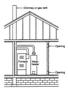
FIGURE 7-1 All Combustion Air from Adjacent Indoor Spaces Through Indoor Combustion Air Openings. [NFPA 54:A.9.3.2.3(1)]
