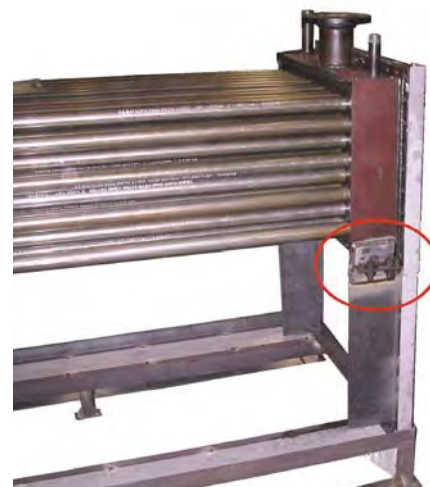
Fig. 4 View of tubes and rear header box showing right side lineal slide assembly.
